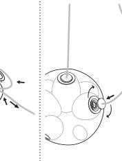
Prior to connecting the remaining tubes to the pendants, be sure to install the glass moons, one moon per tube.
