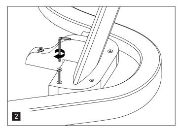
Tighten each screw firmly, but avoid overtightening. Be careful not to scratch the leg with the hex key.
